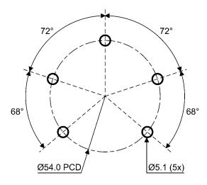
The sensor should be fitted with a gasket if the SAE 5-bolt installation method is used. Fit the gasket over the bolts, black face up, and tighten the bolts to a torque of 10 Nm each.
