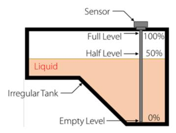
In this situation, 50% of the tank volume is not half way up the probe. To correct for this tank profiling can be used. This can be done in the GSlevel software and is covered in detail in the GSlevel User Manual.
